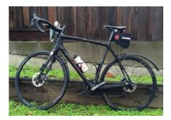
Now, would I consider disc brakes for a bike normally not ridden in the rain? No. I have all the stopping power I need from my rim brakes, and that dry stopping power of a rim vs disc brake isn't much different, if at all. Plus the extra weight of a disc brake, and finally, the annoyance of a bit of pad drag on the rotor (noise, which tries to convince you that you're wasting a lot of effort, which you aren't).
